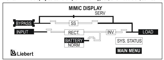
In this example, the power is coming from the bypass source through the bypass switch to the load. The UPS module is off, as shown by the open rectifier and inverter switches. Notice also that the battery circuit breaker is open.
